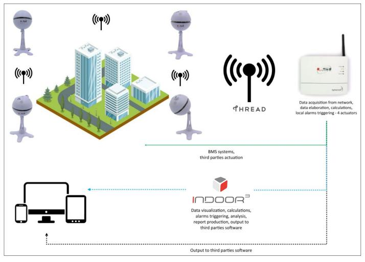
The **Sphensor** data logger sensors form an indoor sensor network and communicate with each other and with the Sphensor Gateway via **2.4 GHz radio**, **Thread protocol**. The Sphensor Gateway (TXRGB1101) with **dual antenna** can receive signals from sensors that communicate on the **868 MHz frequency**.
