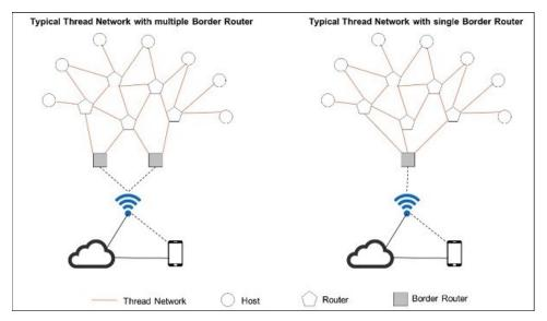
▶ The **Thread protocol** allows the connection and communication of the Sphensor<sup>TM</sup> data logger sensor network to one or more Sphensor Gateways.
