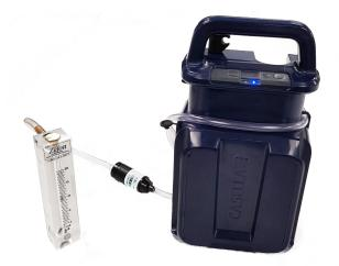
Our air sampling family is complete. With a low-flow (VAPex), medium flow (Apex2) and high-flow (Vortex3) pumps available!
